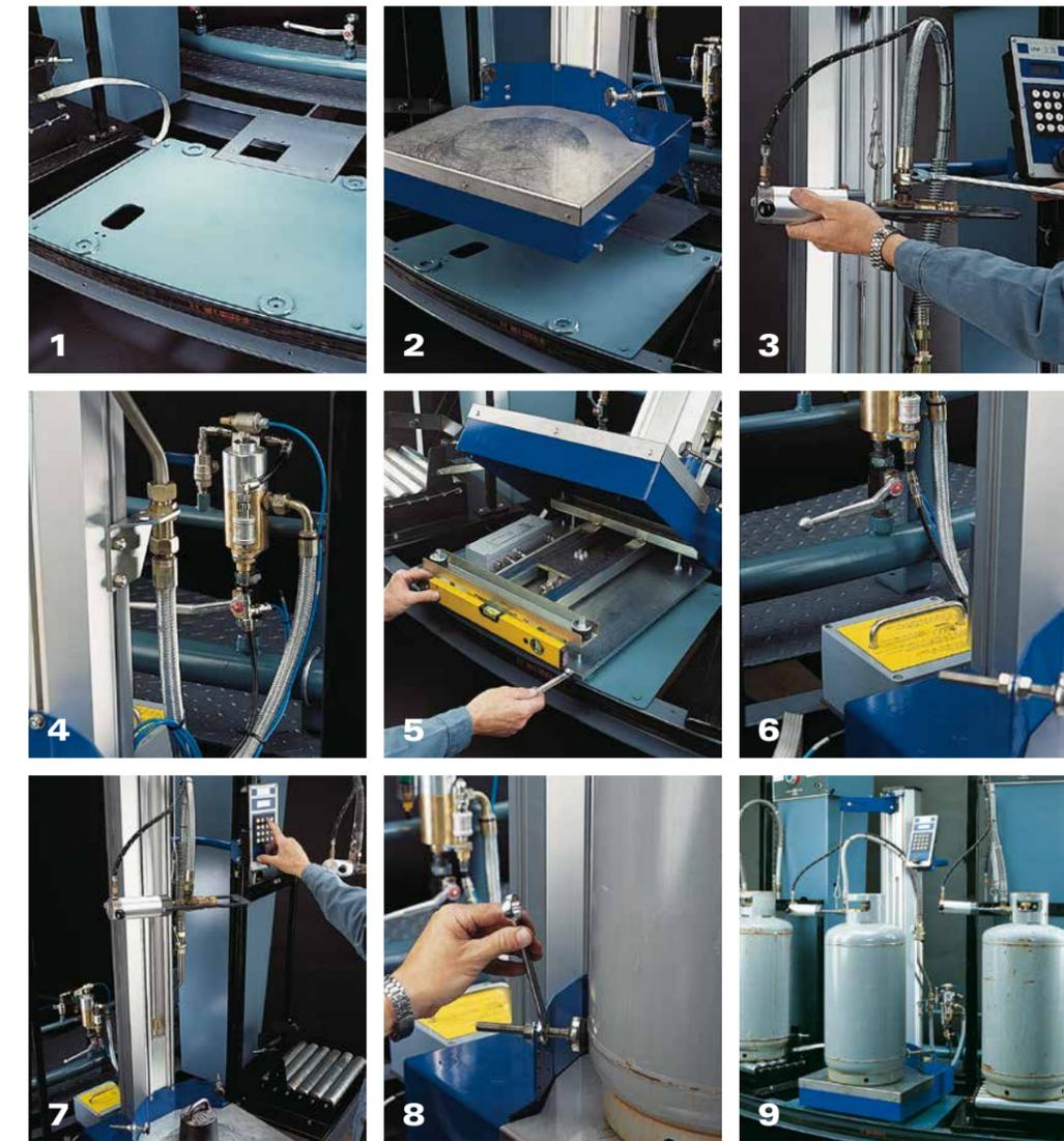
(1) After dismantling the filling machine to be replaced, a customer-designed adapter plate (included in the supply) is mounted on the carousel.
